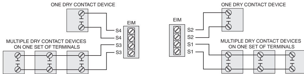
Fig. 157. Wiring dry contact devices.
