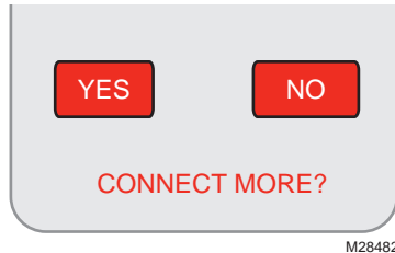
Fig. 47. Connect additional thermostats to Portable Comfort Control.
